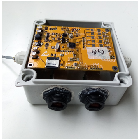
Figure 7. The ARM-Node inside IP67 enclosure. The rugged RJ45 connectors and cable glands are shown.
