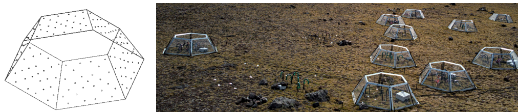
Figure 1. Visualization of an OTC chamber used in the experiments in order to simulate the day time warming and a photograph of a measurement spot (King George Island, South Shetlands), with OTC installed.
