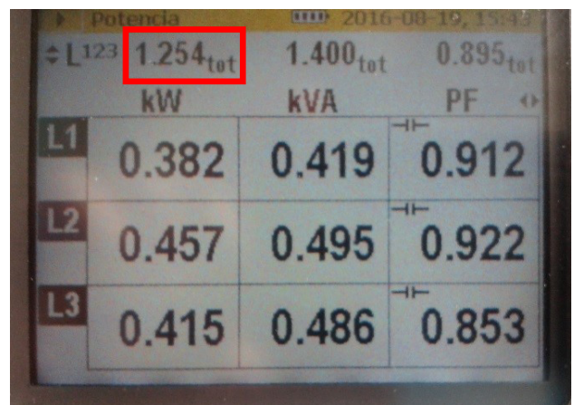
FIGURE 14. Active/apparent power and power factor once the alternator is connected to the grid.
