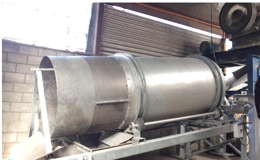
Fig. 1. Crushing machine used for collection HCP from demolished concrete wastes.
