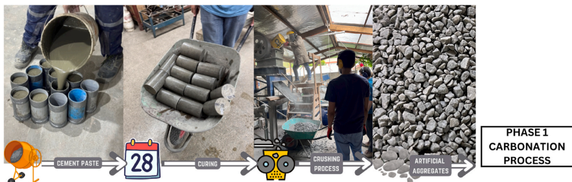
Fig. 2. Manufacture of cement paste aggregates.
