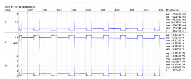
FIGURE 11. Current (top), voltage (middle) and power (bottom) waveforms for a 10min test without applying the strategy for reduced energy consumption.
