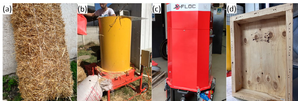
Figure 1. Wheat straw in bales (a), biomass grinder equipment (b), blowing machine (c), test specimens for blowing the material (d).
