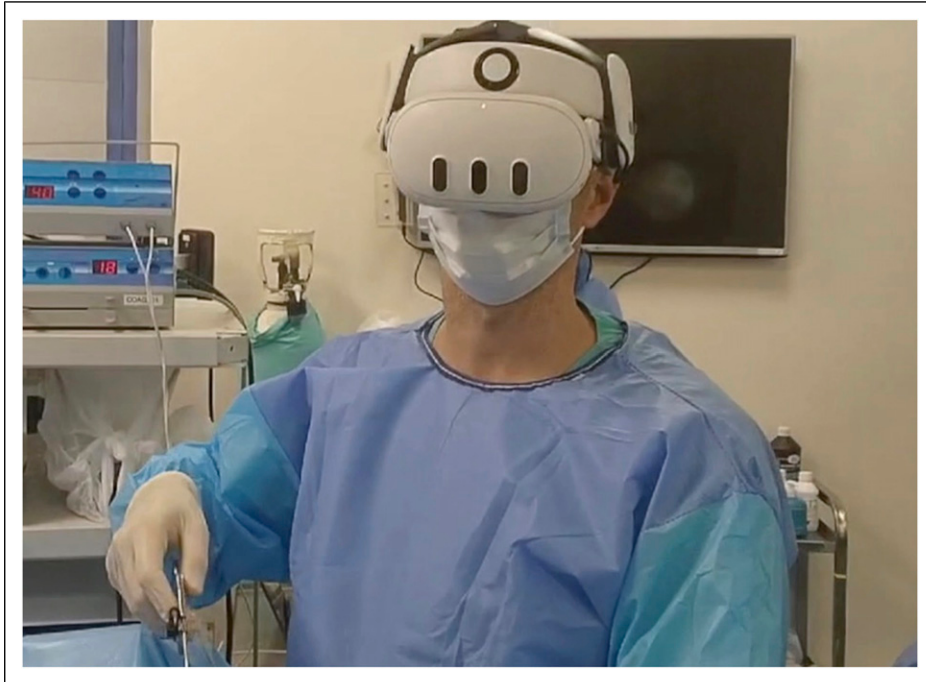
Figure 2. Intraoperative Use of the AR System. Note that the Surgeon's Neck and Head Can Remain Neutral and Relaxed or Be Adjusted Without Relying on Physical Monitors
