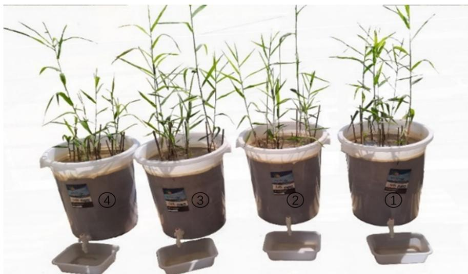
**Figure 2.** Simulated constructed wetland devices (from right to left, wetlands No. 1, 2, 3, and 4).
