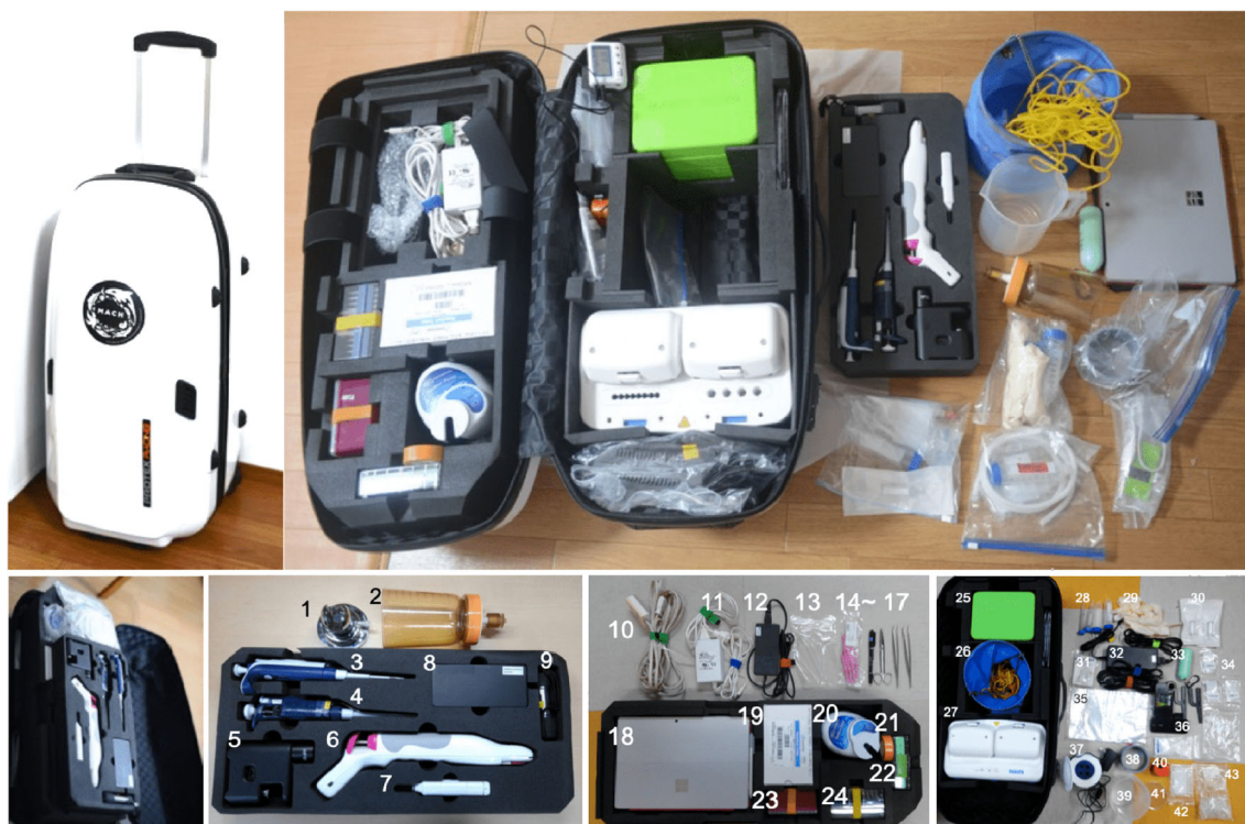
Fig. 1 The Suitcase Lab. The Suitcase Lab is 47 × 39 × 90 cm (W × D × H) and weights 15 kg. It contains 43 tools
